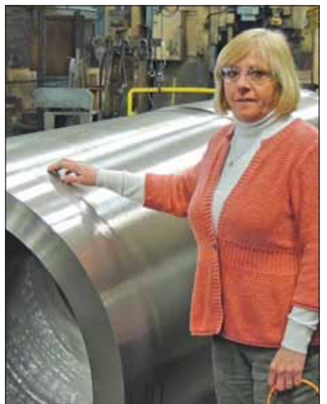
Becky Monahan with a finished paper dryer canister, built at GL&V in Hudson Falls for a paper mill. Chronicle photo/Gordon Woodworth
